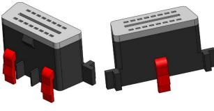
remove the plastic lugs marked red (e.g. witch a sharp knife)
